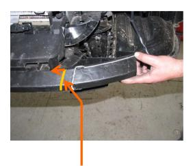
Trim both ends of air dam 30mm from plastic web at arrow point. This dimension is a little wider than the distance between the bullbars' alloy mounting brackets.
