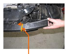
Trim both ends of air dam 30mm from plastic web at arrow point. This dimension is a little wider than the distance between the bullbars' alloy mounting brackets.
