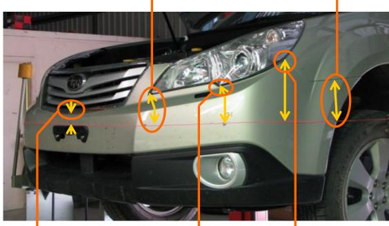
NOTE: Dimensions correct for current model- file photo from previous model24 mm from bottom edge of chrome-<br/>work surround-<br/>ing grill145 mm from headlight
