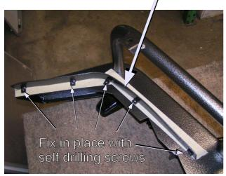
\* Trim off approx 10-15mm from front 3 edges of plastic sumpguard, so as to make front edge straighter when looking from side of vehicle. This is to allow front edge of sumpguard to fit into protector.
