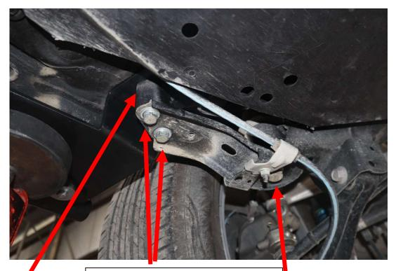
Subframe spacer be careful to leave this in the correct position. Remove the two 12mm subframe bolts and slot bracket between chassis and subframe or subframe spacer, these will be 14mm bolts if you have a lift kit installed
