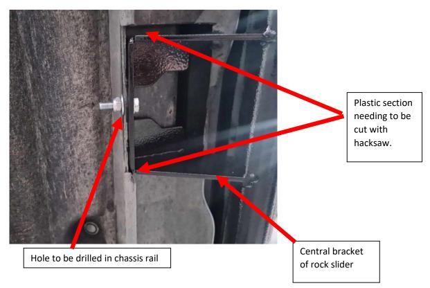
3. You will need to trim a small rectangular section out of the plastic cladding to allow for the central rock slider bracket to be mounted to the
