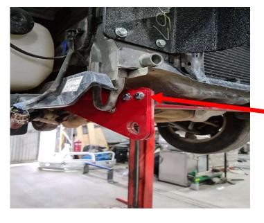
3 x M8 x 30mm bolts and nyloc nuts mentioned in step 3
