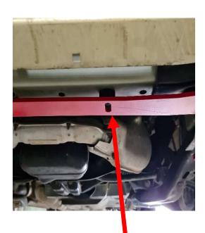
Aluminium spacers fit here between red part and chassis
