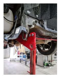
Slide the recovery point centre section into the middle of each of the side section's. Using 3 x M8x30mm bolts, Nyloc nuts and matching washers on each side, loosely bolt the centre recovery section and the side plates together.
