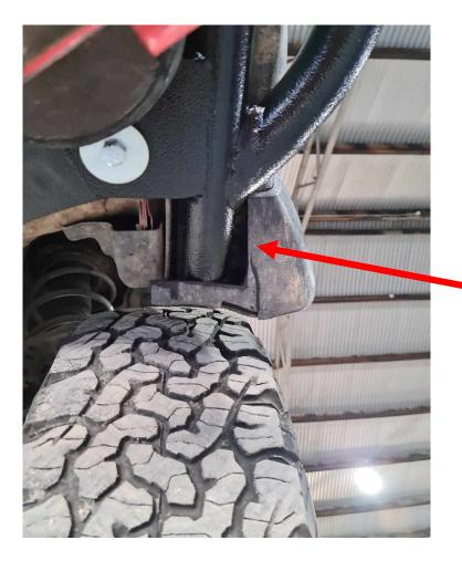
Rectangular section cut from the mudflap to allow rock slider enough room to fit.
