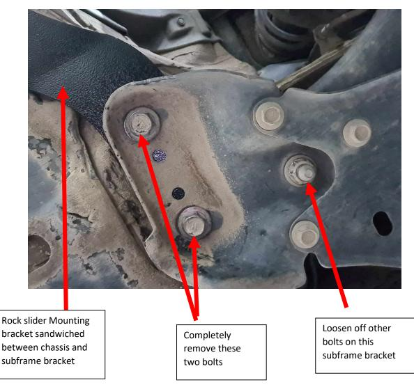
4. To install the front Rock slider bracket, similar steps as with the rear mounting bracket will be followed. As seen in photo above, completely remove the two indicated bolts from the subframe mounting bracket, loosen the rest of the bolts holding this subframe bracket to the chassis,. Slide the rock slider bracket between the subframe bracket and the chassis sandwiching them together.
