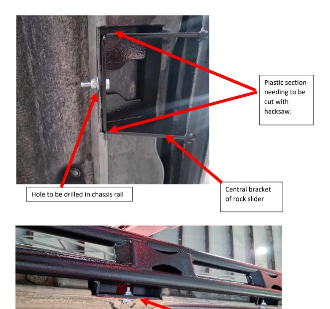
3. You will also need to remove the factory mudflaps from the front wheel arches, there is one clip and two screw holding this part on. There is some trimming required of the Mudflap, a picture of the modification is below.
