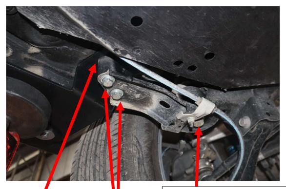
Loosen rear bolt on bracket, this bolt must be re bolted to Torque spec the correct specifications are 107ft/lb or 145NM
