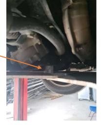
5. Using two M8x 35mm bolts and two large panel washers attach the front of the sump guard to the vehicle, adjust and then tighten all bolts.
