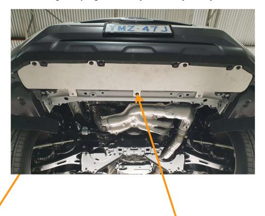
Use clips from engine shield to hold shield in place
