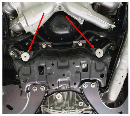
5. Place sumpguard in position seen below. Using 2 supplied M8x35mm bolts and washers, loosley fit the bolts to the rear of the transmission bracket first.
