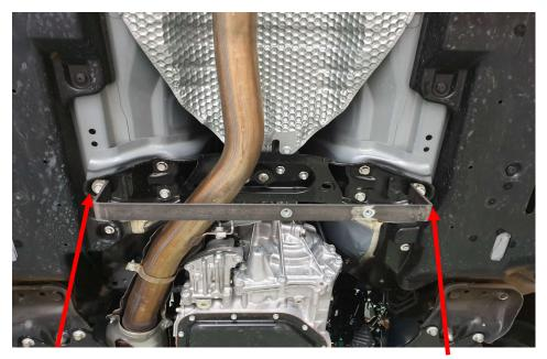
Remove the 2 outer crossmember bolts then fit back in when bracket is in place.
