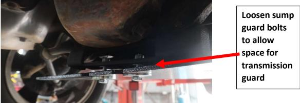
2. Using the factory subframe bolts that are already in the space, Mount the smaller rear transmission bracket into the gap shown in the photo below with the subframe bolts. Make sure to mount the bracket in the correct direction with the angled side of the bracket following the shape of the subframe.
