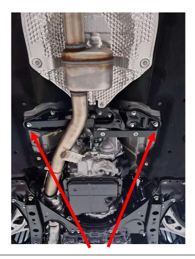
Remove the 2 outer crossmember bolts then fit back in when bracket is in place.
